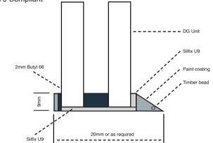
N&C Eco-lite™ Slim comes in a range of finishes, available for renovating or the restoration of period properties. Each option offers a reduced sightline & manufactured as a traditional hermetically sealed unit.
